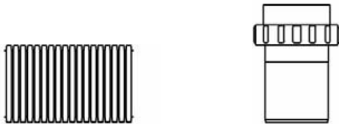
Figure 6 – Conduit flexible et raccord flexible / rigide
